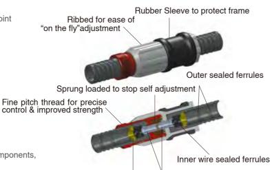
Brass inserted ferrules Lined Aluminum internals
