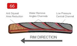
Ashima entry level EBS pad, with advanced groove profile: inspired by a car tire tread the central channel that runs the entire length of the brake surface, ensures contaminates have a low pressure escape route away from the brake/rim interface, giving superior wet performance.
